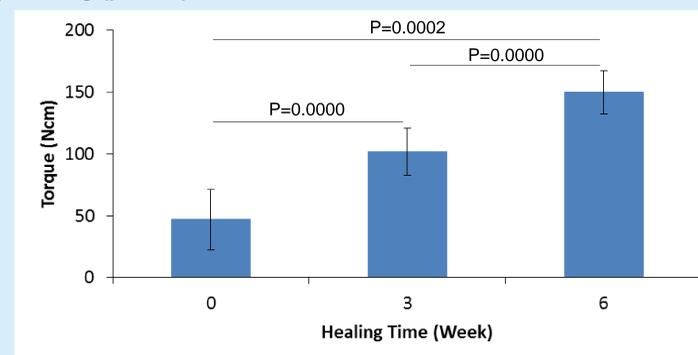
Figure 3. Maximum torque values at placement, 3 and 6 weeks. RTV at 3 and 6 weeks were significantly higher than ITV at implant placement (p<0.05). From 3 weeks to 6 weeks of healing, RTV increased significantly (p<0.05).
