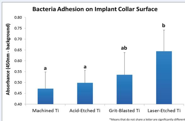
**Figure 2.** Bacteria adhesion on implant collar surfaces. Implant collars were incubated in bacteria-containing broth for 24 h. Following, the total amount of bacteria that adhered to each surface was quantified.
