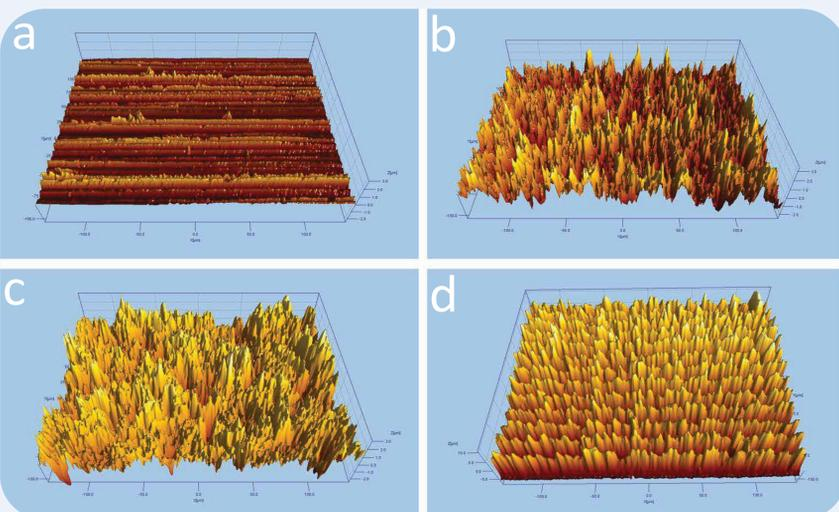
**Figure 1.** Interferometry maps of implant collar surfaces. A surface mapping microscope was used to quantify the roughness of (a) machined, (b) acid-etched, (c) grit-blasted, and (d) laser-etched titanium surfaces.
