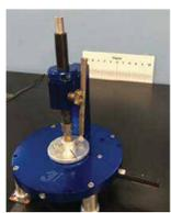
Figure 1. Abutment Angular Rotation (AAR) equipment measured the degrees of clockwise and counterclockwise rotation the abutment can withstand when seated on the implant.
