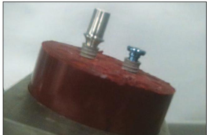
**Figure 2:** Representative implant mounted with 3.0mm simulated resorption.
