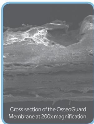
Cross section of the OsseoGuard Membrane at 200x magnification.
