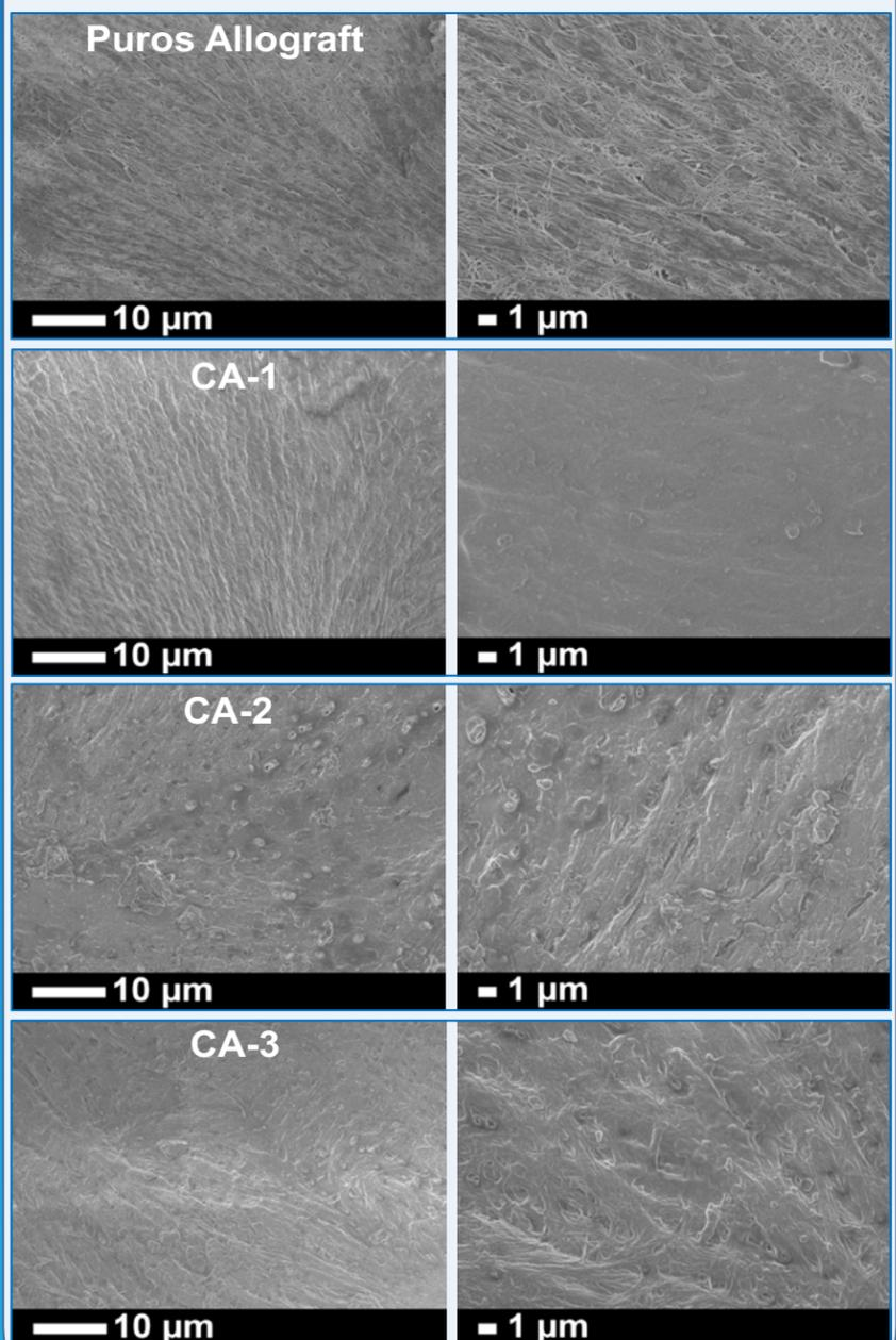
Figure 4. Field-emission scanning electron microscope images indicated porous surface structure of Puros allograft.
