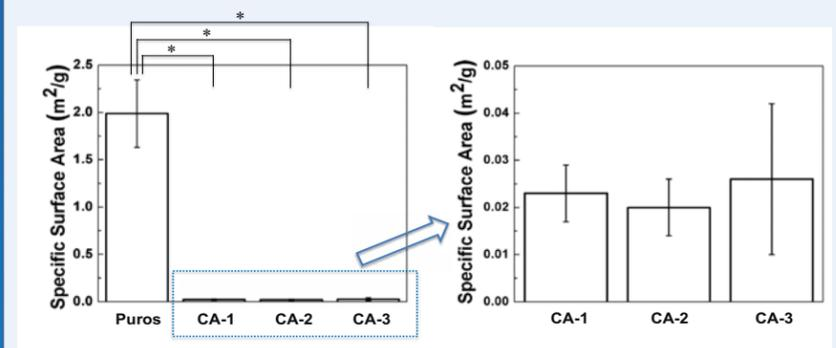
Figure 3. Surface area comparison from BET analysis. Puros allograft exhibited two orders of magnitude higher specific surface area as compared to other allografts, which confirmed the porous structure of Puros allograft.
